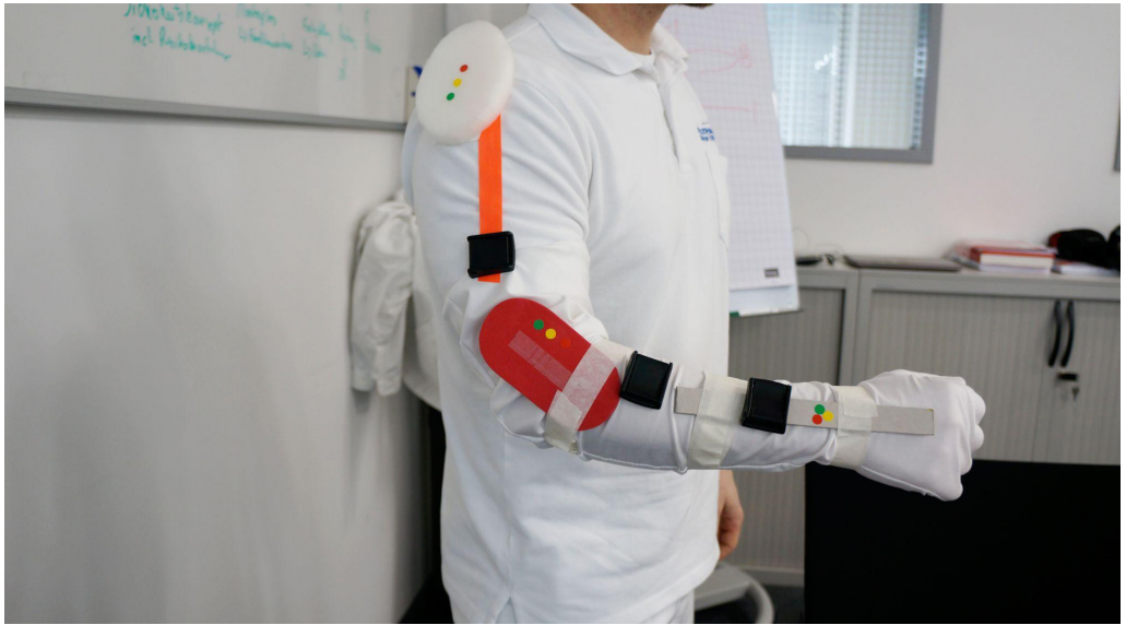
Figure 2.2. Lo-fi prototype of a wearable soft robotic orthosis for communicating needs and requirements during a workshop with users. Note: From “Designing a Wearable Soft-Robotic Orthosis: A Body-Centered Approach” by R. Flechtner, K. Lorenz, and G. Joost, in Proceedings of the Fourteenth International Conference on Tangible, Embedded, and Embodied Interaction (TEI '20) (p. 867), 2020, Association for Computing Machinery.
