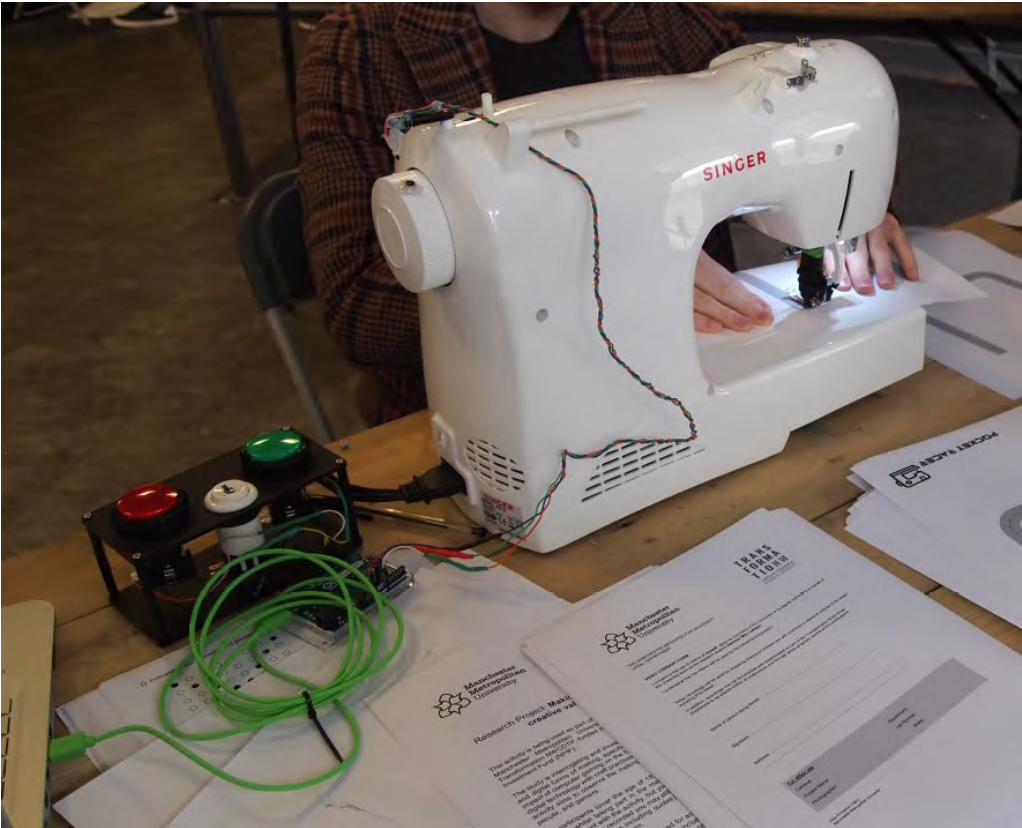
Figure 4.4. Participant interacting with Pocket Racer , including a sewing machine with a sensor positioned above the handwheel, an external Arduino, and accept/reject buttons.
