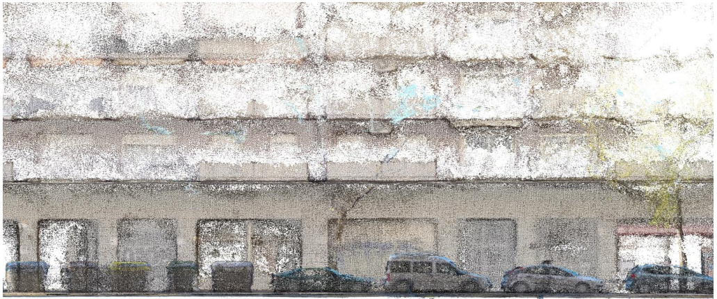
Figure 12.2. Point Cloud reconstruction of Consell de Cent, Barcelona.
