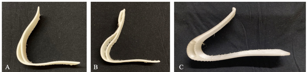
Figure 10.2. A: 3D printed heel arch. B: heel arch iteration with strap mounts and pre-tension. C: 1:1 scale prototype of the final heel arch 3D printed in flexible PLA to be fitted in the shoe.
