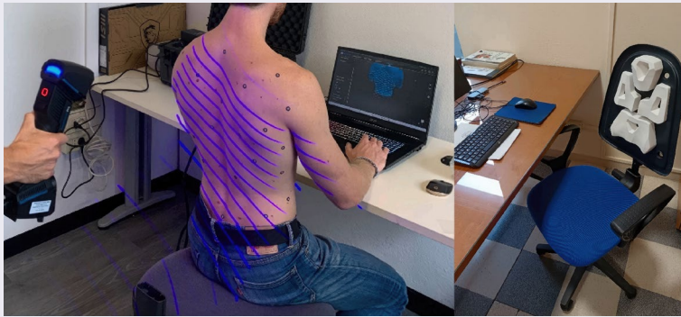
Figure 4. Scanning process and 3D printed backrest. Credits: Pagliari et al. , 2025.
