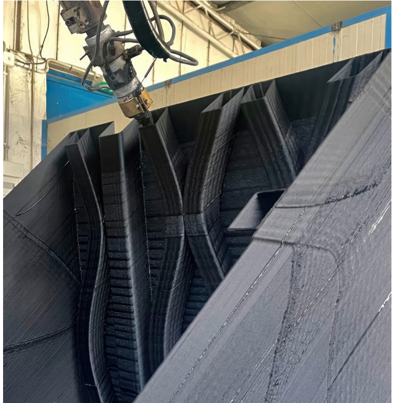
Figure 19. Prototype during the 3D printing process, showing the robotic arm extruding the material layer by layer.
