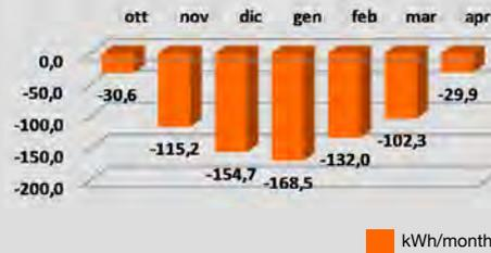
**Evaluation of energy performances of passive solar greenhouse of building with 4 cm of insulation**
