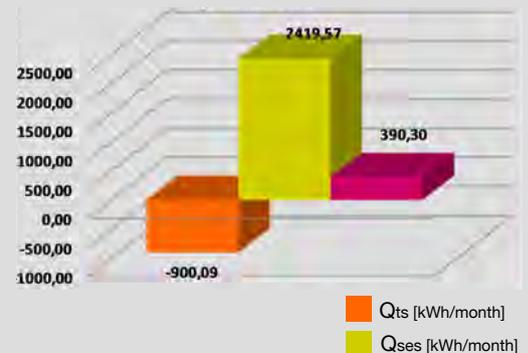
**QSE,S : Assessment of the amount of solar energy due to greenhouse being adjacent to heated spaces**
