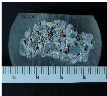
Fig. 08 : Cross section of a mortar from Barbarossa walls (sample 2)
