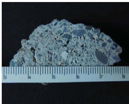
Fig. 12 : Cross section of a bedding mortar from the XVI th century rampart of the fort near Porta Siberia (s. 10)
