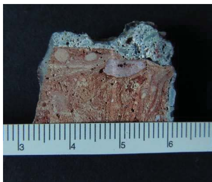
Fig. 16 : Cross section a brick from the corner of a rampart of Sperone Fort (sample 17)
