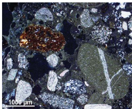
Fig. 09 : Thin section of sample 2 (image at the optical microscope in transmitted polarized light-XPL)
