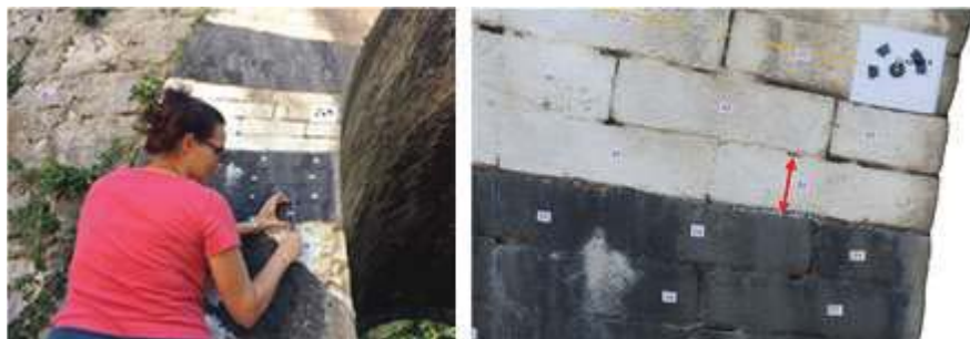
Fig. 02 : Case A. On-site measurement with caliper, and tiled view of the underpass 3D model with marked bricks for measurement test; operators agreed to measure near the marked number
