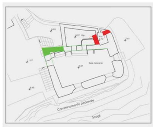
Fig. 04 : Belforte planimetry with the location of the wall transformations: the red walls were demolished to enlarge the fort, the green wall is the new one
