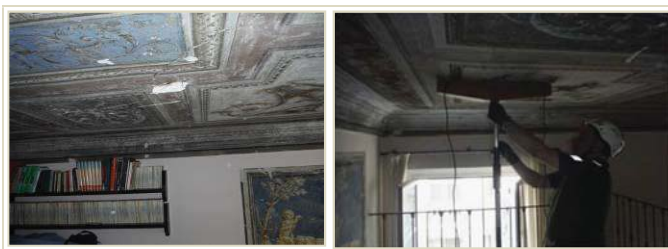
Figg. 05-06 : Image of the ceiling in wattle and of the ultrasonic test
