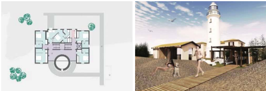
Figg. 05/06 : Goro Lighthouse: reuse general plan, first floor. Right: a project rendering: the lighthouse with the proposed removable wooden structure as seen from the seaside
