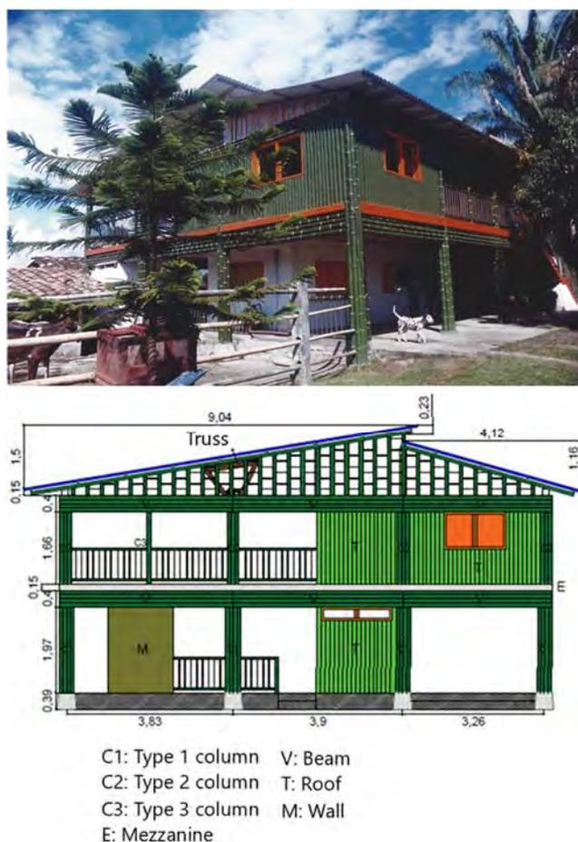
Fig. 2 – (a)Housing case study (b). Diagram of the cross-sectional view of the dwelling
