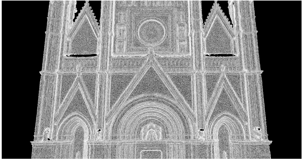
Fig. 4. Polygonal mesh returned by Metashape.
