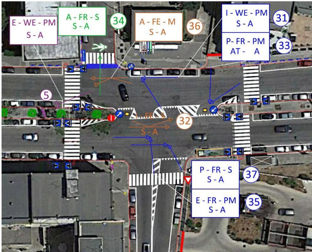
Fig. 14.51: Detailed Collision Diagram - Intersection IV (photo source Google Earth).
