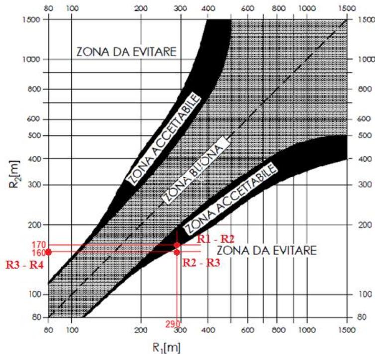
Fig. 13.14: Abacus n.5.2.2.a, D.M. 11/05/2001<sup>9</sup> (“Zona da evitare” = unacceptable ratio between two subsequent curves, “zona buona” = good ratio, “zona accettabile” = acceptable ratio).
