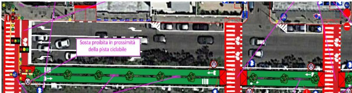
Fig. 14.54: Long-term countermeasures T1 - Northern part (Sosta proibita in prossimità della pista ciclabile = prohibited parking next to the cycle lane).
