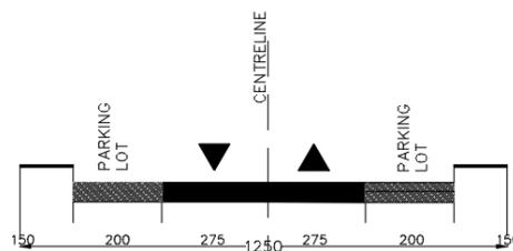
Fig. 14.27: Standard cross section of the F category road according to D.M. 6792/2001<sup>3</sup>.
