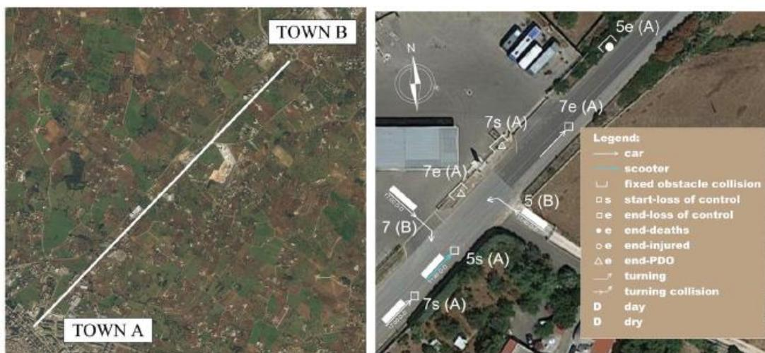
Fig. 13.28: Horizontal alignment and collision diagram of the example road segment characterized by many accesses and minor intersections (Colonna et al., 2018<sup>5</sup>).
