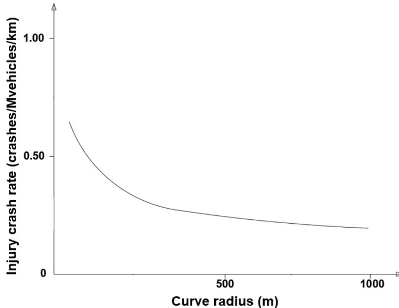
Fig. 3.13: Relationship between radius of curvature and injury crash rate (based on Elvik and Vaa, 2004<sup>59</sup>).
