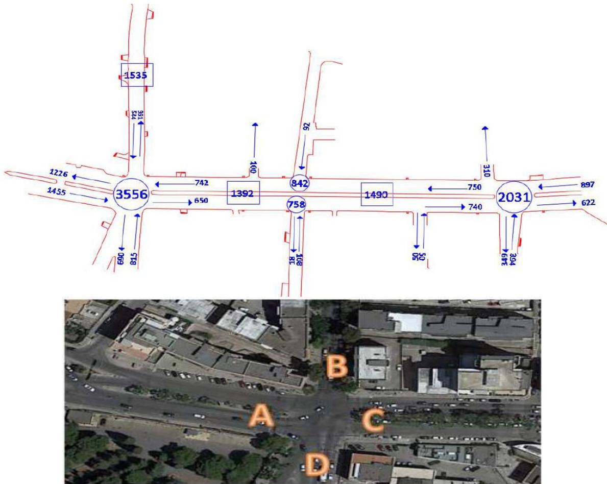
Fig. 14.44: Map of traffic flows assigned to segments and intersections (and legend of the directions used for the O/D matrix).
