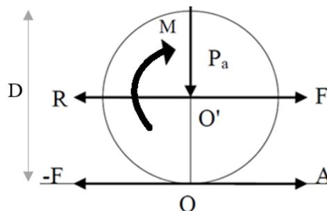
Fig. 9.2: Forces acting on the wheel.
