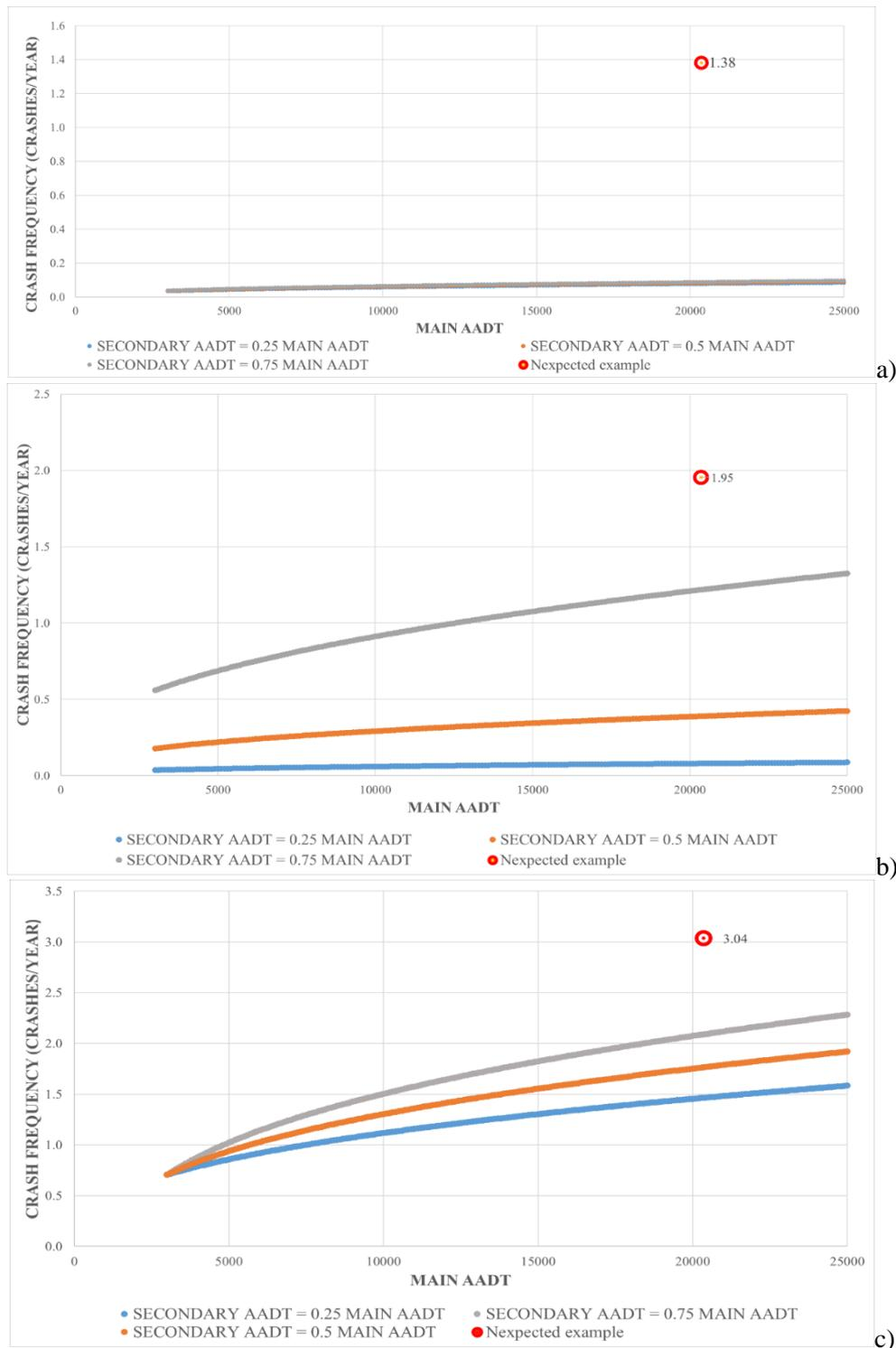
Fig. 14.2: Comparison of the  $N_{expected}$  calculated for the example of application with some SPFs developed by a) Gomes et al. (2012)<sup>1</sup> for 4-legged intersections, b) Intini et al. (2020)<sup>2</sup> for signalized intersections, c) Intini et al. (2020)<sup>2</sup> for 4-legged intersections. See chapter 14.10 for more information about those SPFs and reference studies.
