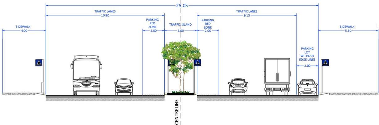
Fig. 14.20: Cross section, section S - S'; road segment of Viale Papa Giovanni XXIII.
