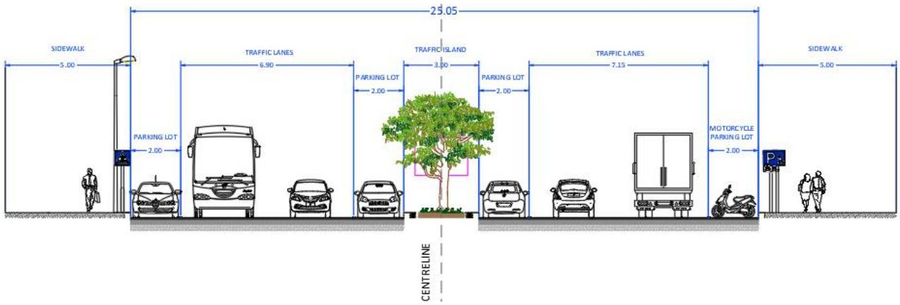
Fig. 14.18: Cross section, section Q-Q'; road segment of Viale Papa Giovanni XXIII.
