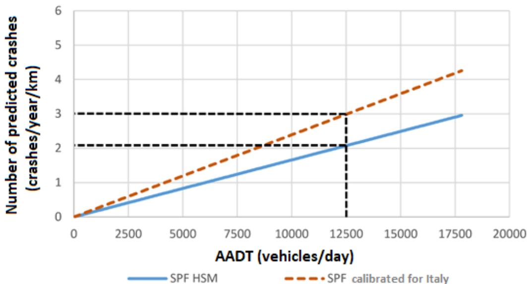
Fig. 12.1: Comparison between HSM base and calibrated SPFs for Italian two-lane rural roads (based on Colonna et al., 2016<sup>6</sup>).
