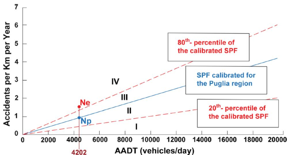
Fig. 13.3: Levels of Service of Safety for two-way two-lane rural roads in the Apulia region with indication of the number predicted by the SPF and expected number of crashes for the site under examination (Colonna et al. 2018<sup>5</sup>).
