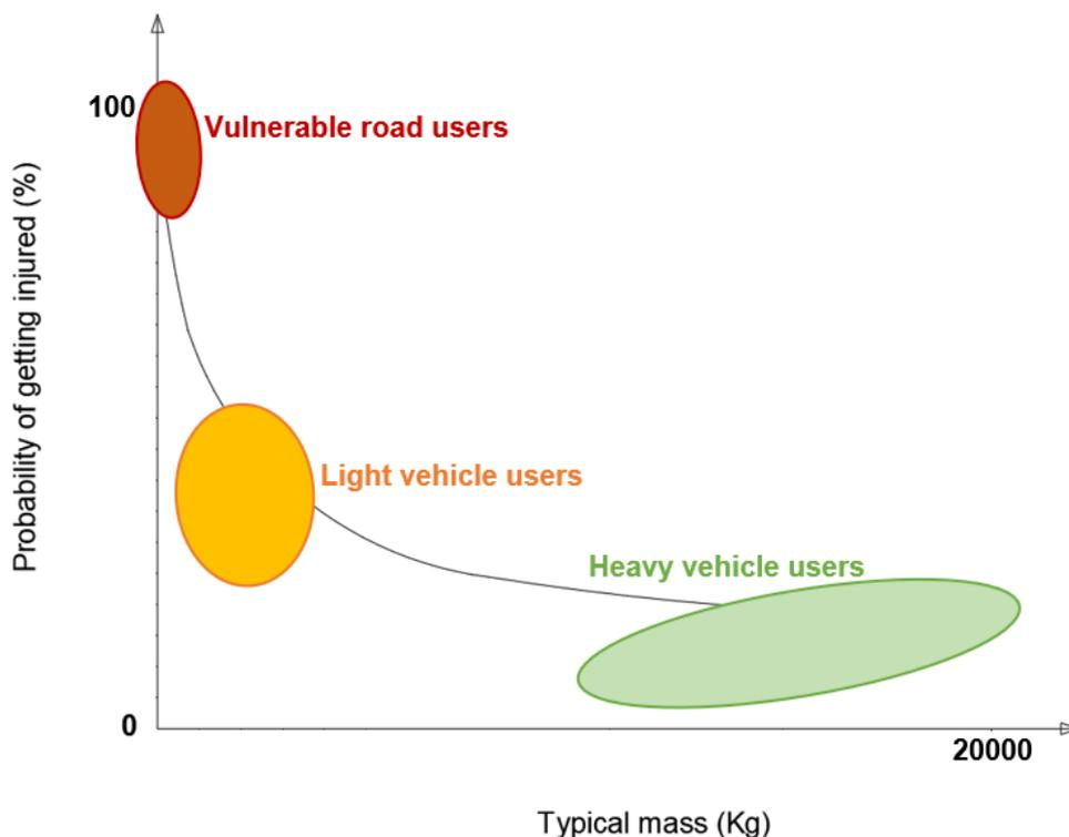
Fig. 3.14: Relationship between accident probability and vehicle type (based on Elvik and Vaa, 2004<sup>59</sup>).
