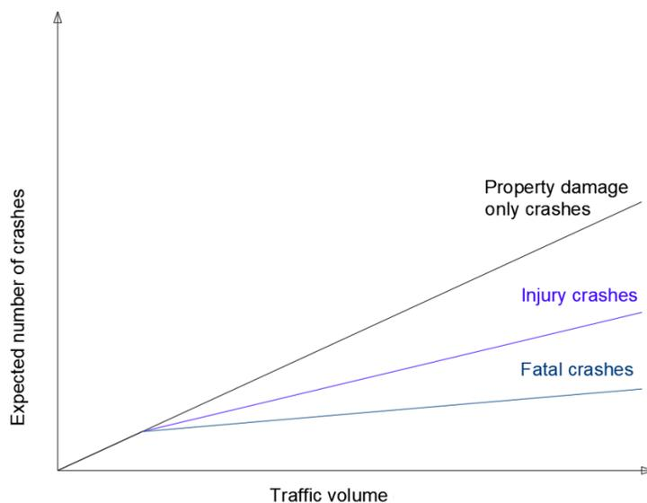
Fig. 3.12: Typical relationships between traffic volume and expected number of crashes (based on Elvik and Vaa, 2004<sup>59</sup>).
