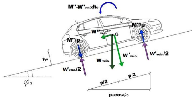
Fig. 9.6: Equivalent static scheme of an uphill vehicle (based on Colonna et al., 2015<sup>5</sup>).
