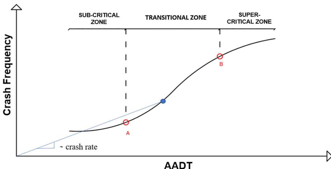
Fig. 10.3: Sub-critical, critical and super-critical zones (based on Kononov et al., 2011<sup>6</sup>).
