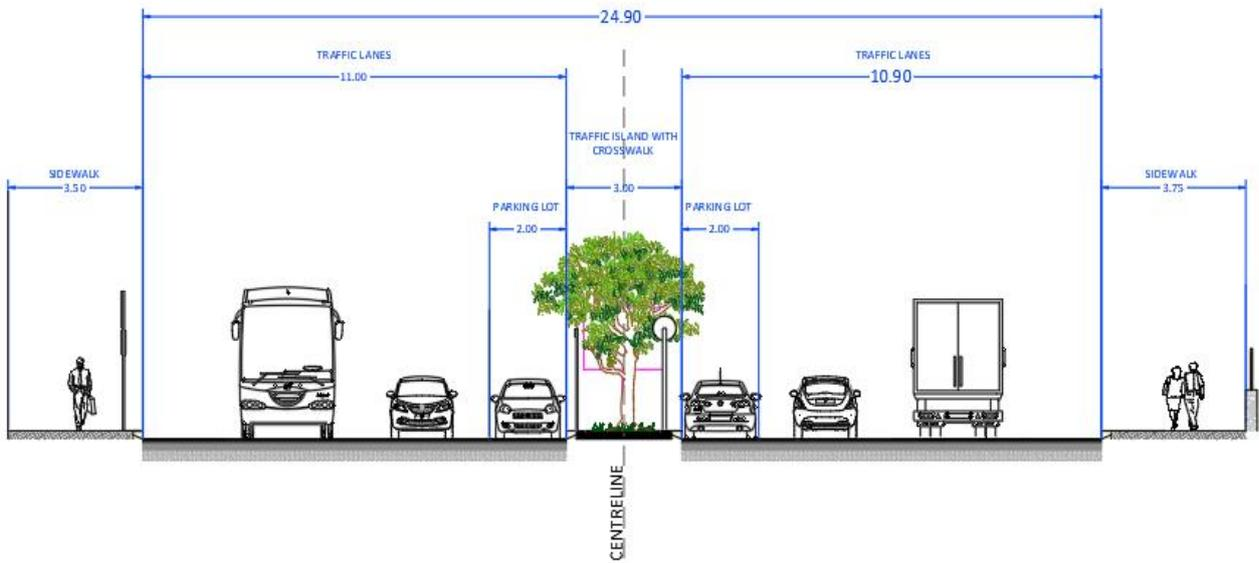
Fig. 14.16: Cross section, section G-G', intersection II and III - Viale Papa Giovanni XXIII.
