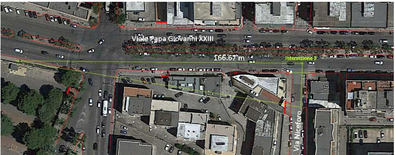
Fig. 14.42: Intersection III Visibility triangles (photo source Google Earth).
