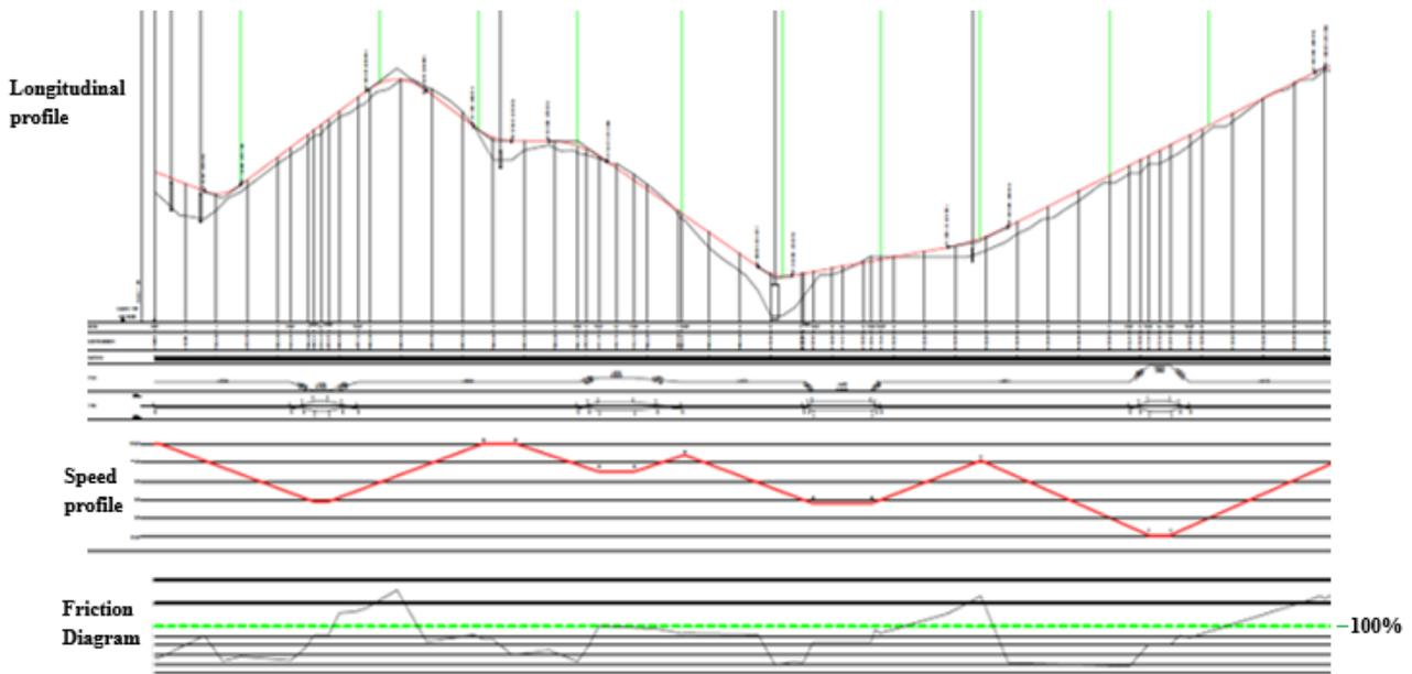
Fig. 9.16: Friction Diagram of the road segment belonging to the SP239, from the km 6+000 to the km 8+000.
