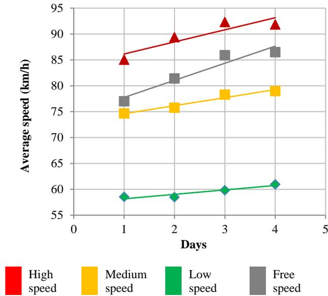
Fig. 4.4: Speed differences between drivers who have acquired route familiarity (fourth day test) and drivers who are initially unfamiliar (first day test) – Results for different speed tasks (based on Colonna et al, 2016<sup>16</sup>).
