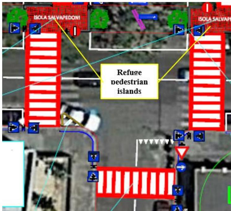
Fig. 14.78: Short-Term countermeasures Intersection III (isola salvapedoni= pedestrian refuge island).
