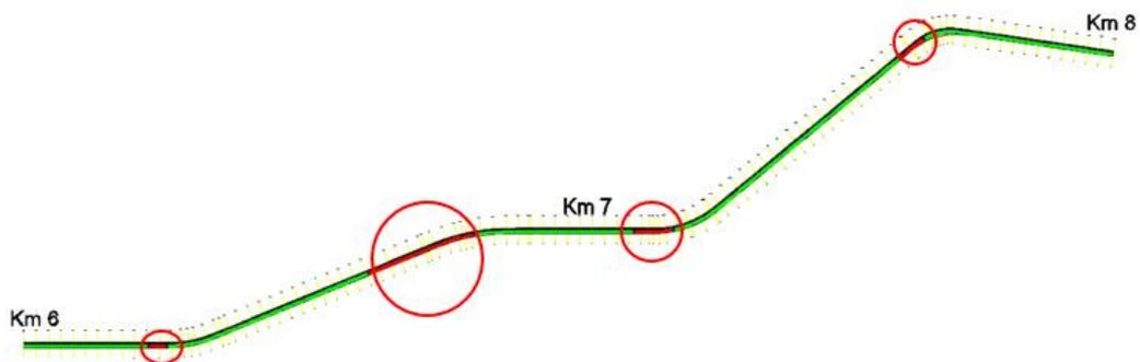
Fig. 13.17: Checks about the stopping sight distance (direction: Noci).
