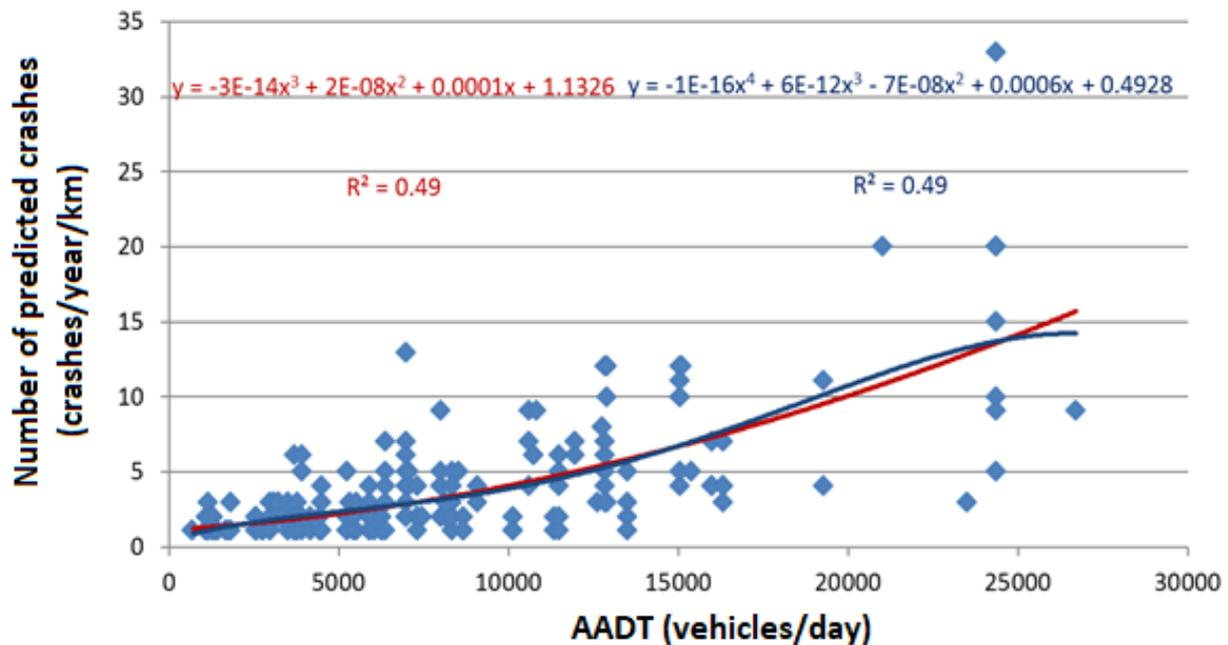
Fig. 12.2: Example of native SPF development with different functional forms.
