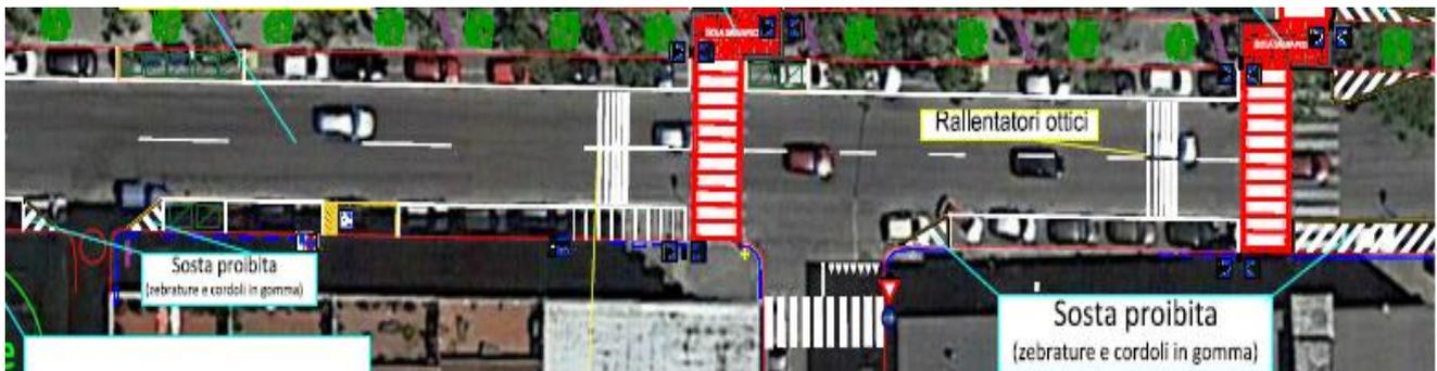
Fig. 14.62: Short-term countermeasures T2 - Southern part” (Sosta proibita = prohibited parking/zebrature e cordoli in gomma = Zebra patterns and rubber kerbs).
