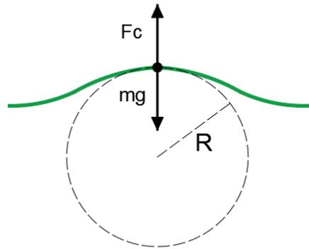
Fig. 9.7: Forces acting on a crest curve.
