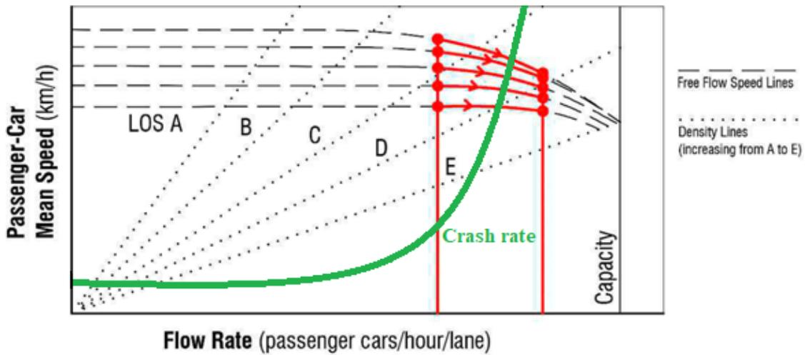
Fig. 10.5: Overlap between the speed-flow-density/LOS curve and the crash rate curve (based on Kononov et al. 2012<sup>7</sup> and HCM (2000)<sup>9</sup> for the LOS concept).
