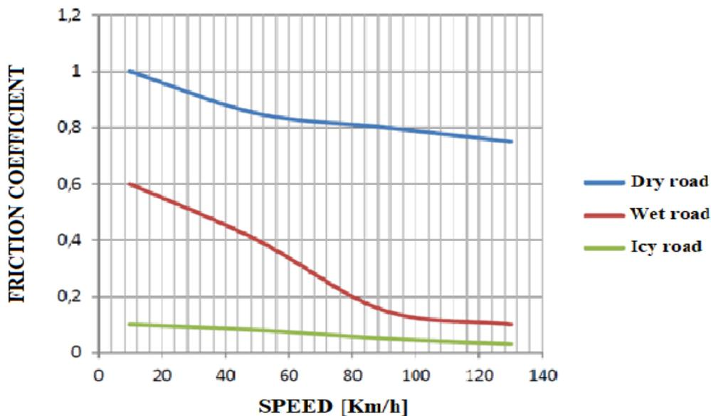
Fig. 13.24: Speed - Friction coefficient diagram.
