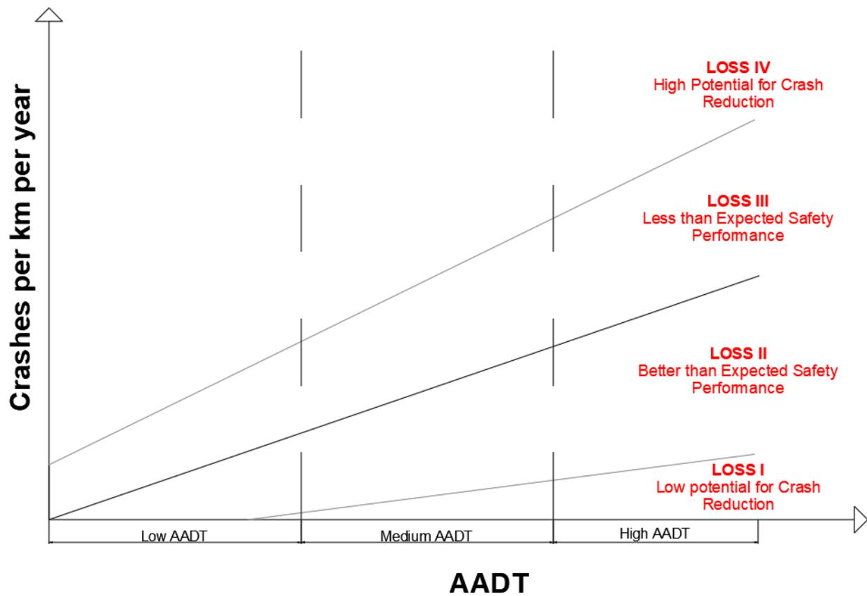
Fig. 10.7: Combination of LOSS areas and AADT ranges for diagnostic purposes (Based on Kononov et al., 2003<sup>4</sup>).
