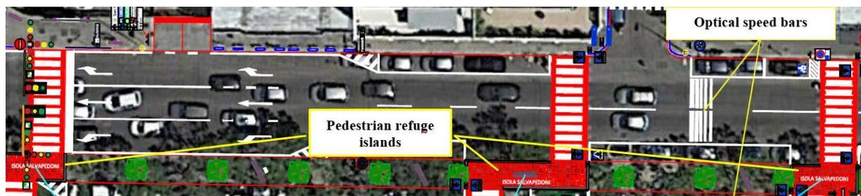
Fig. 14.53: Short-term countermeasures T1 - Northern part (transverse optical speed bar and pedestrian refuge islands).
