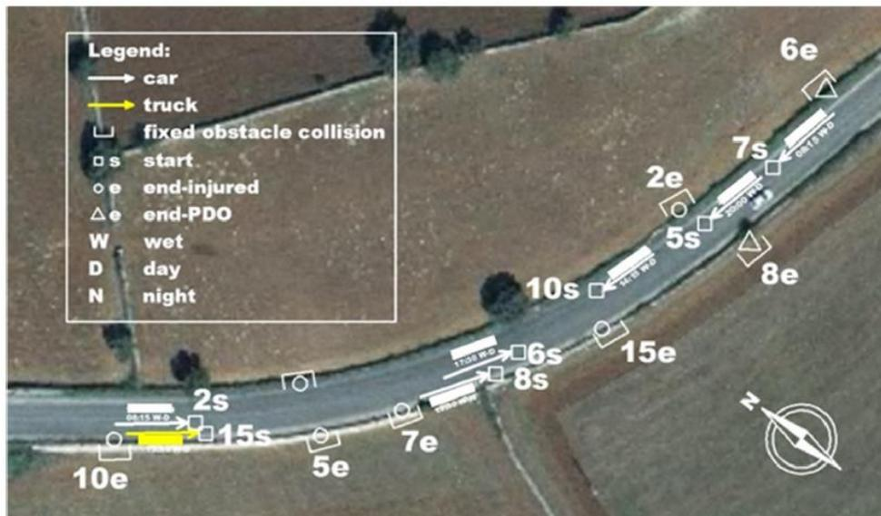
Fig. 13.7: Example of Collision diagram- Curve 3 (Colonna et al., 2018<sup>5</sup>).
