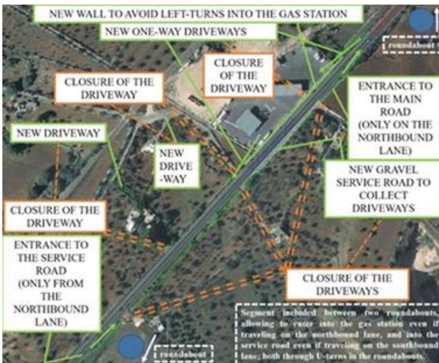
Fig. 13.30: Example of secondary roads for the collection of flows from minor intersections (Colonna et al., 2018<sup>5</sup>).
