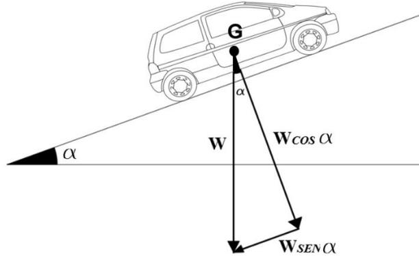
Fig. 9.3: Adherent weight of a vehicle on an uphill road.
