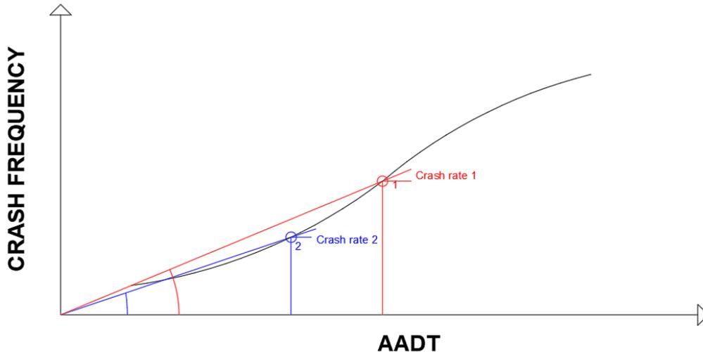
Fig. 2.1: Example of Safety Performance Function (based on Kononov and Allery, 2003<sup>3</sup>).
