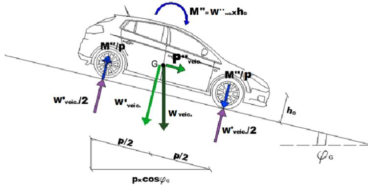
Fig. 9.5: Equivalent static scheme of a downhill vehicle (based on Colonna et al., 2015<sup>5</sup>).
