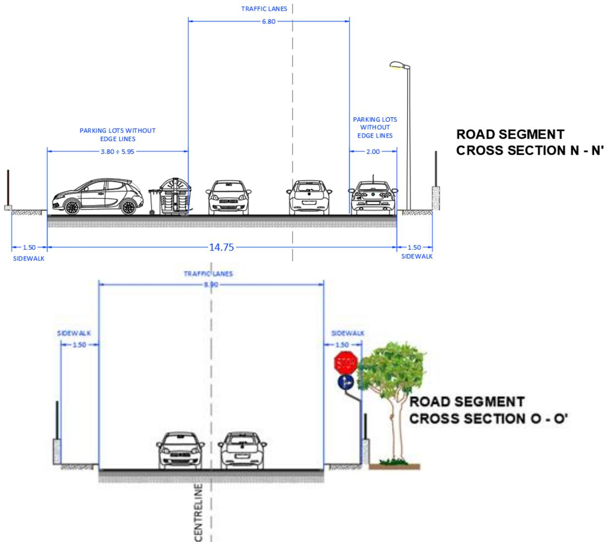
Fig. 14.26: Cross section, road segment sections – Via Niceforo.
