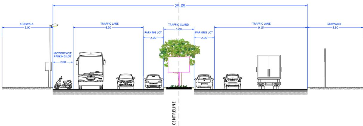
Fig. 14.19: Cross section, section R - R'; road segment of Viale Papa Giovanni XXIII.
