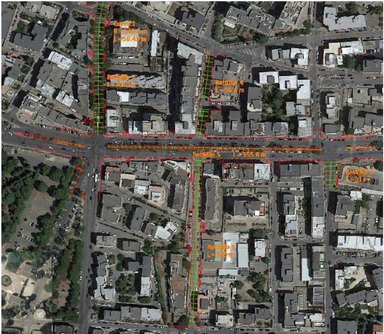
Fig. 14.11: Whole reconstruction of the road curbs and centerlines of the analysed area (photo source Google Earth).
