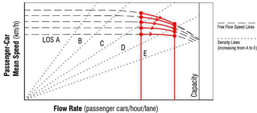
Fig. 4.2: Example of effects of increasing the equivalent flow rate on the level of service (taken from Intini, 2017<sup>25</sup>, based on the Highway Capacity Manual, 2010<sup>24</sup>).
