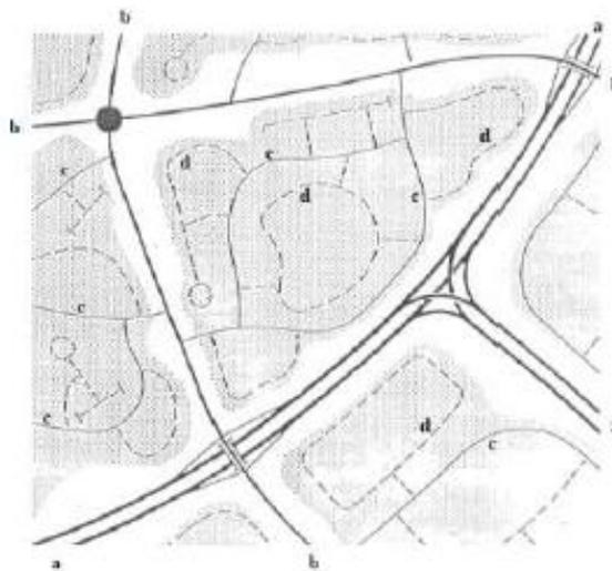
Fig. 14.7: Road network levels according to the D.M. 6792/2001<sup>3</sup>.
