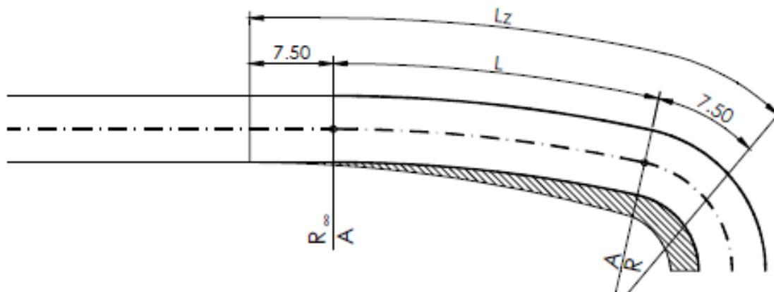
Fig. 13.15: Enlargement at the spiral curve (D.M. 6792/2001<sup>9</sup>).
