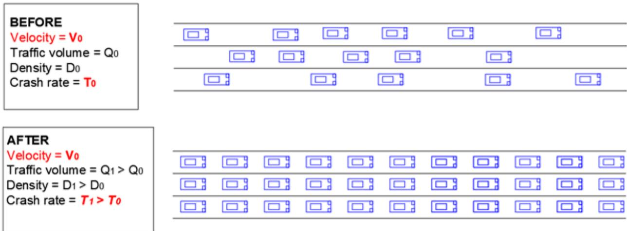
Fig. 10.4: The crash probability, for an equal speed, is higher at higher vehicle densities (Kononov et al., 2011<sup>6</sup>).
