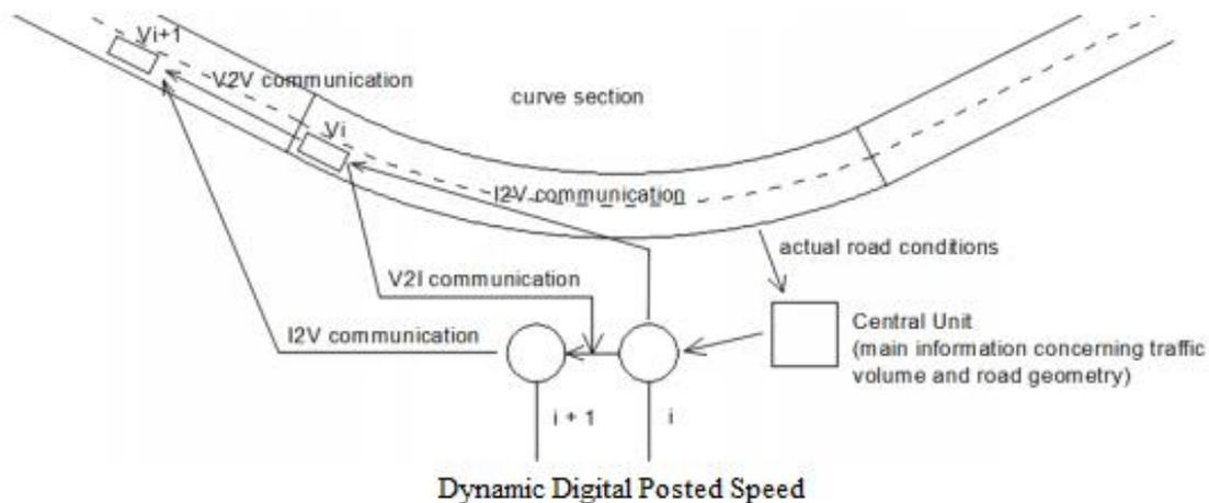
Fig. 9.20: The possible communication system among vehicles, sensors and units, to dynamically determine the posted speeds (Intini et al., 2019<sup>12</sup>).
