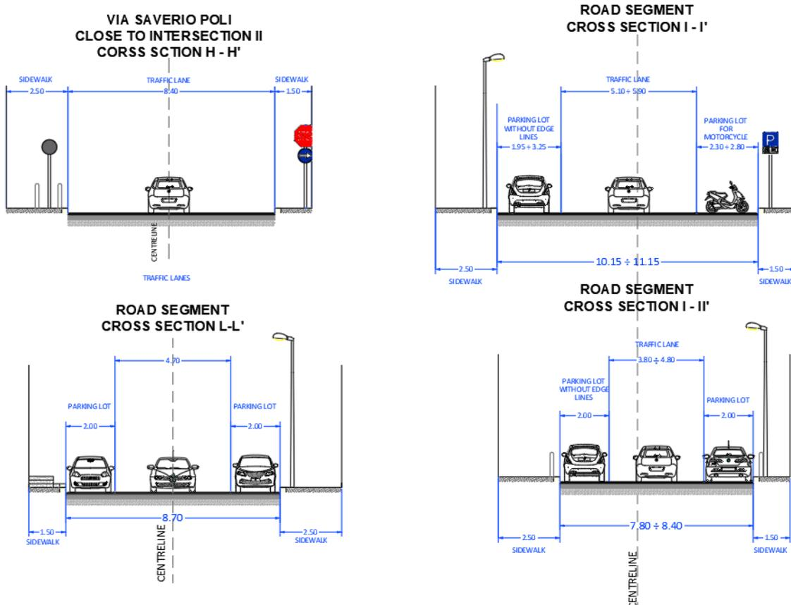
Fig. 14.24: Cross section of Via Saverio Poli.
