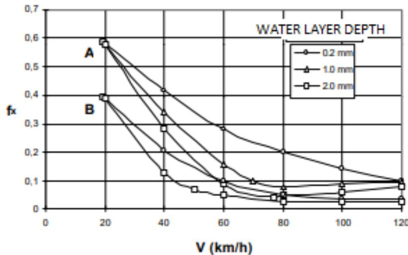
Fig. 9.9: Speed Diagram - Friction Coefficient. The curves show the friction coefficient versus speed if the tyre has the tread (A) or not (B), Canale et al. 1998<sup>6</sup>.
