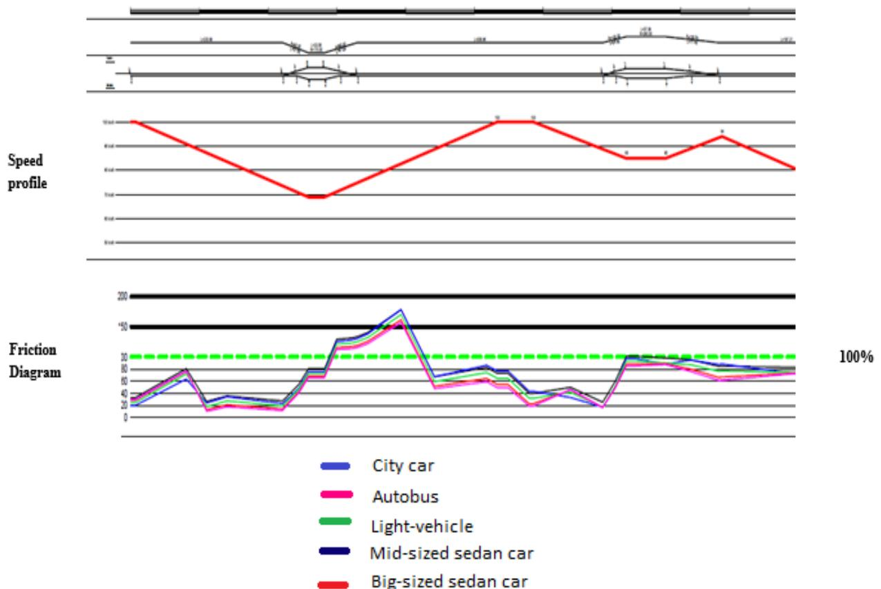
Fig. 9.17: Comparison among Friction Diagrams about the road segment of the SP239, from the km 6+000 to the km 8+000, for different vehicle types. Different colors stand for different vehicles.
