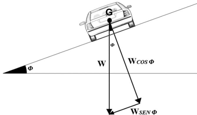
Fig. 9.4: Adherent weight of a vehicle on a road segment with  $\Phi$  cross slope.
