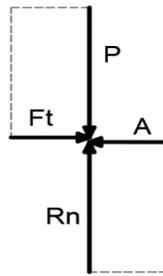
Fig. 9.1: Friction force on a surface.
