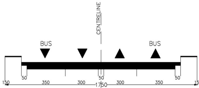
Fig. 14.22: Standard cross section of the “E” category road according to D.M. 6792/2001<sup>3</sup>.
