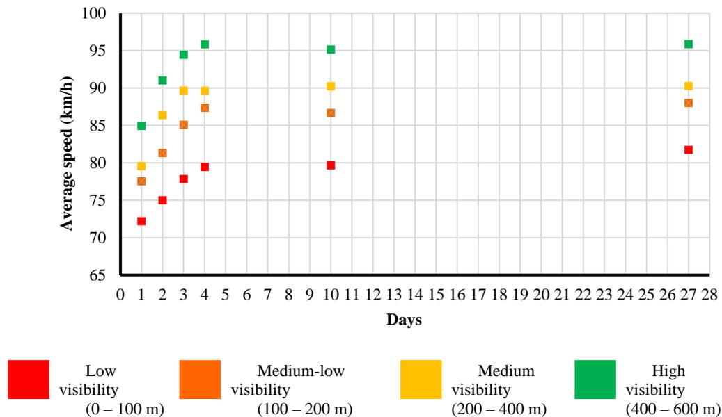
Fig. 4.3: Speed differences between drivers who have acquired route familiarity (fourth day test) and drivers who are initially unfamiliar (first day test) – Results for different visibility classes (based on Colonna et al., 2016<sup>16</sup>).
