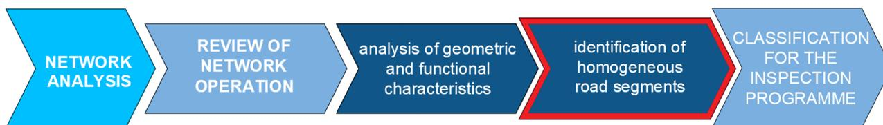
Fig. 5.7: Identification of homogeneous road segments
