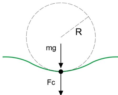
Fig. 9.8: Forces acting on a sag curve.
