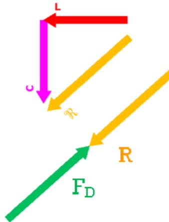
Fig. 9.12: Friction Demand opposing to the sum of all the forces,  $R$ , acting on the vehicle.
