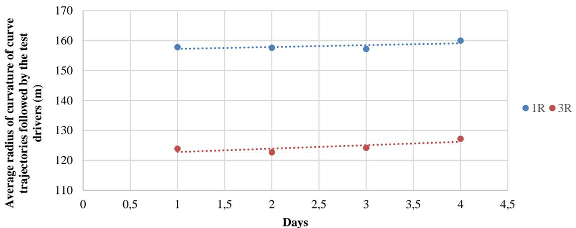
Fig. 4.5: Differences in the radii of curve trajectories between drivers who have acquired route familiarity (fourth day test) and drivers who are initially unfamiliar (first day test) – Results for two test curves (based on Colonna et al., 2016<sup>16</sup>).
