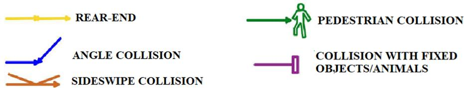
Fig. 14.49: Symbols used in the Collision Diagram (as based on the HSM).
