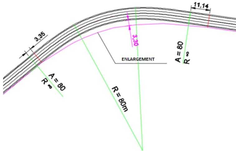
Fig. 13.16: "Curve 4" enlargement.
