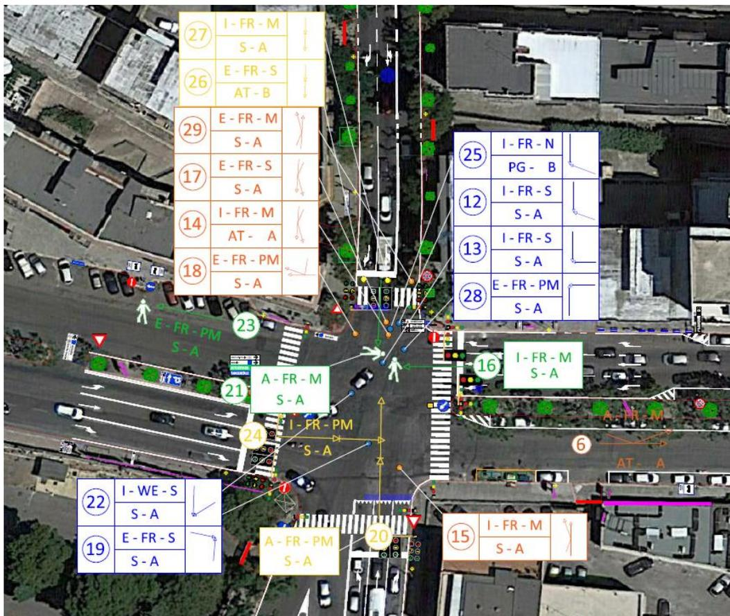
Fig. 14.50: Detailed Collision Diagram - Intersection I (photo source Google Earth).
