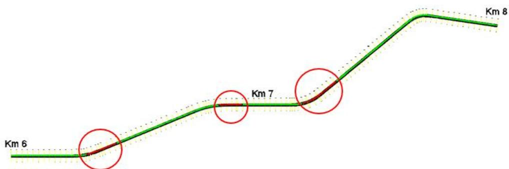
Fig. 13.18: Checks about the stopping sight distance (direction: Gioia del Colle).
