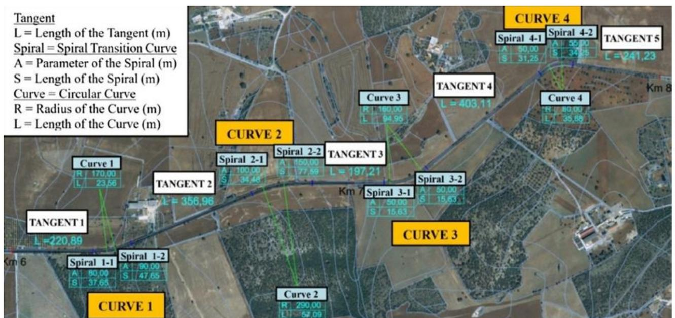
Fig. 13.4: General overview of the analysed segment with division in homogenous parts (Colonna et al., 2018<sup>5</sup>).
