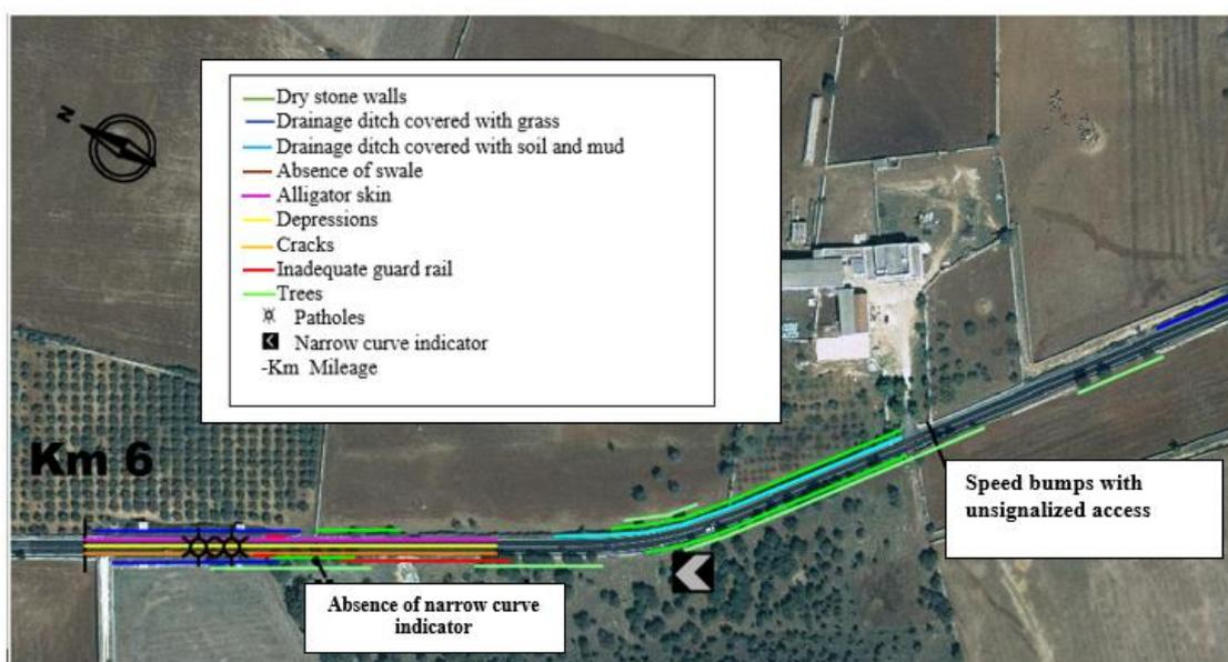
Fig. 13.8: Example of Condition diagram- Curve 1 (Colonna et al., 2018<sup>5</sup>).
