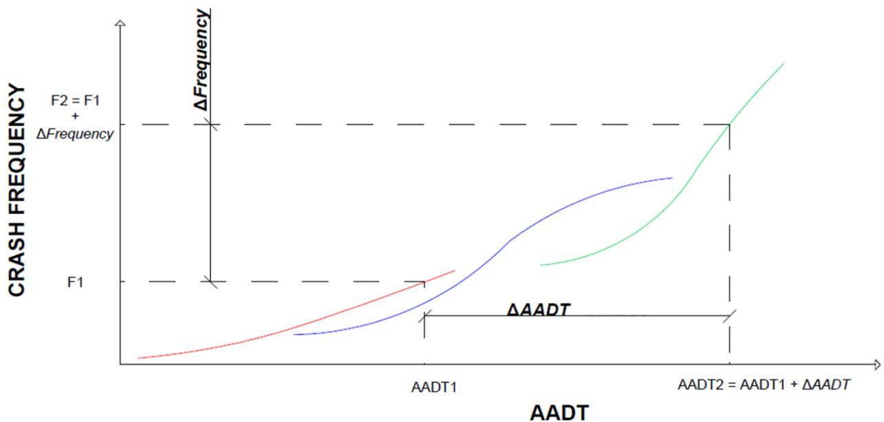
Fig. 10.6: Relationship between crash frequency and number of lanes, from 4-lane freeways (in red) to 8-lane freeways (in green) (based on Kononov et al., 2008<sup>8</sup>).
