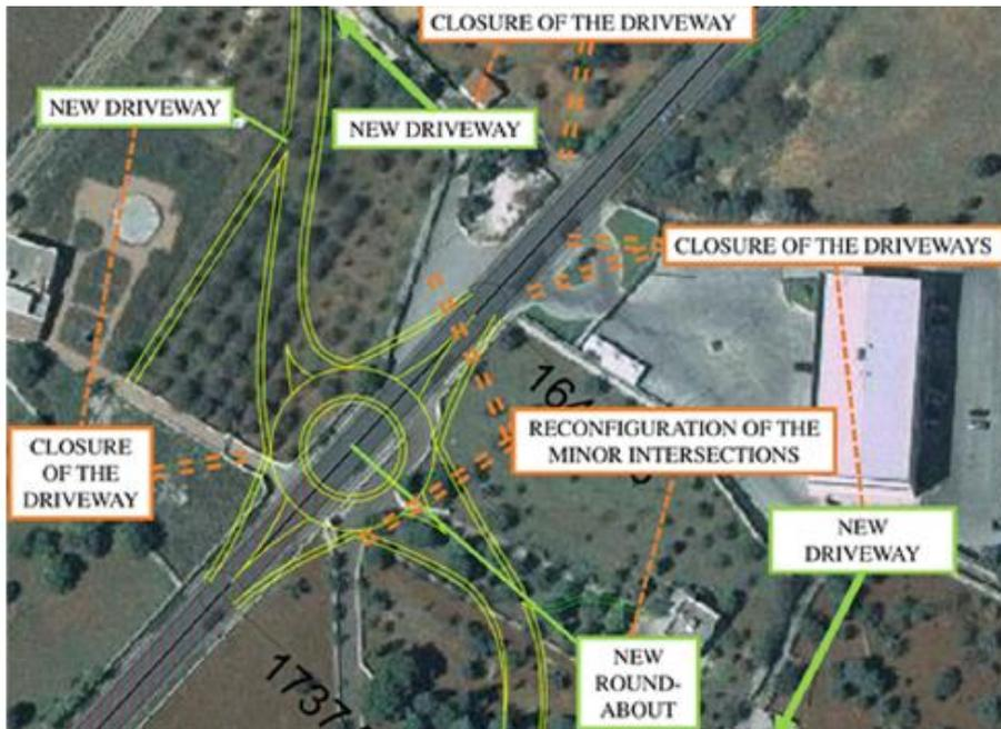
Fig. 13.29: Example of roundabout for enhancing minor intersection geometry (Colonna et al., 2018<sup>5</sup>).
