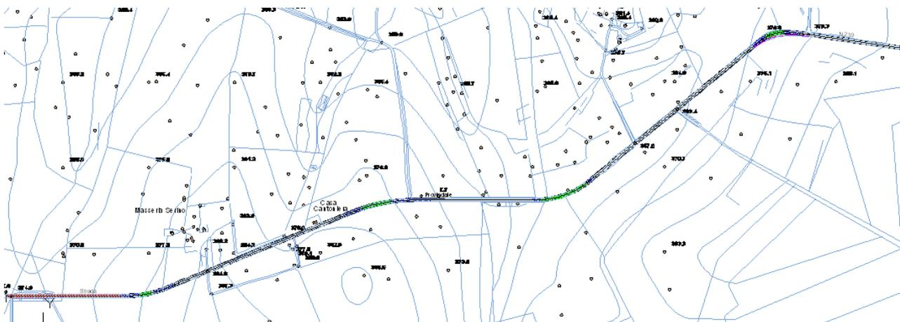
Fig. 9.15: Horizontal alignment on the regional technical map of the analysed road segment (see Chapter 13).
