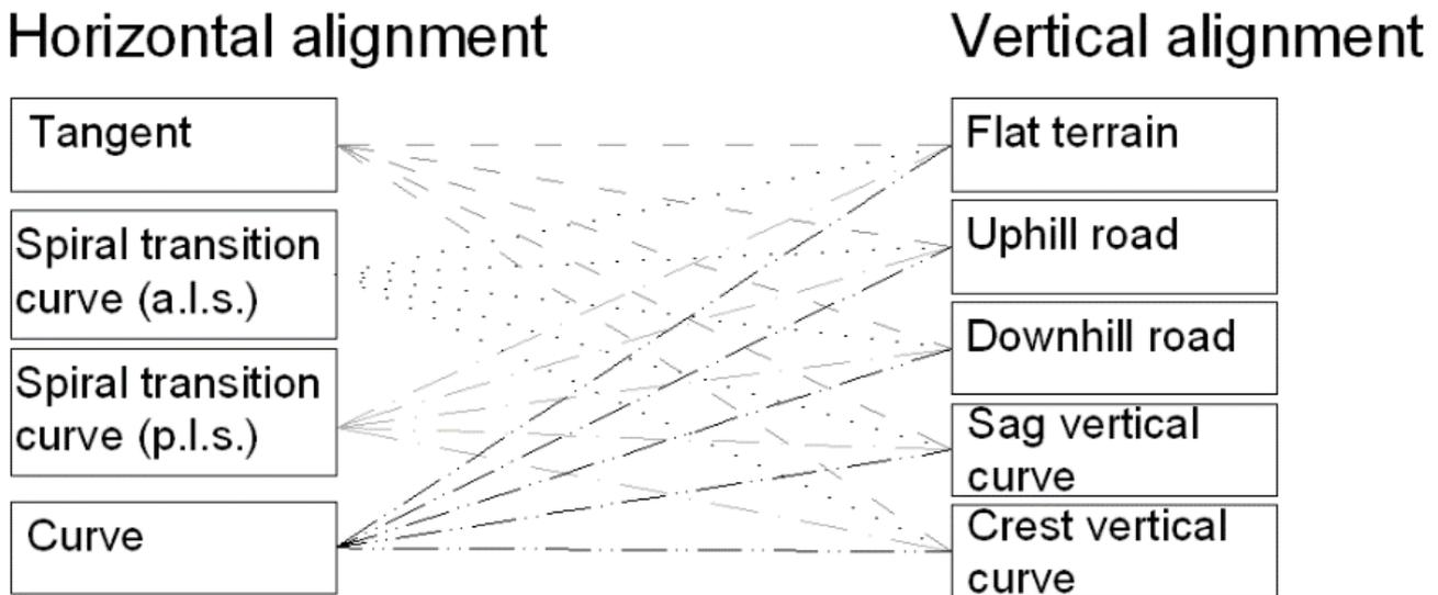
Fig. 9.18: Horizontal-vertical alignment combinations.
