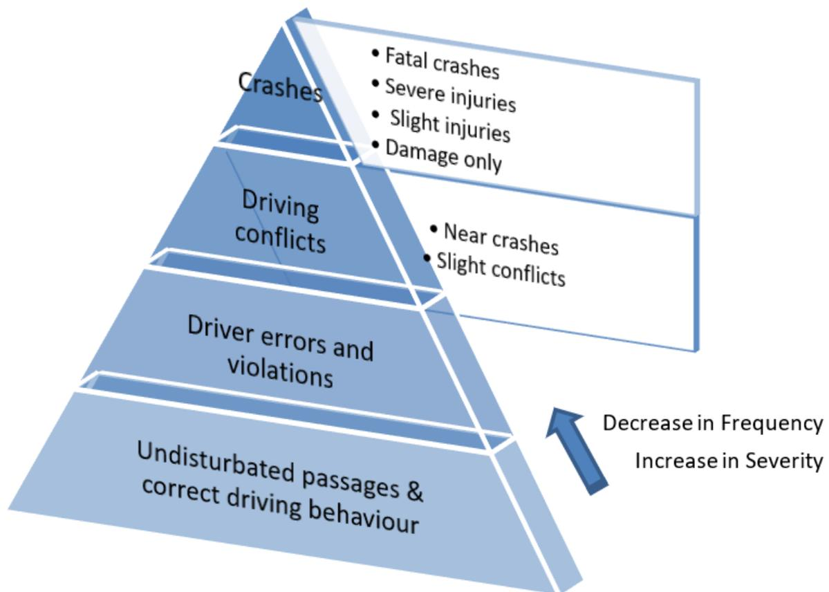
Fig. 3.2: Hayden pyramid (Based on Hayden, 1987<sup>18</sup>).
