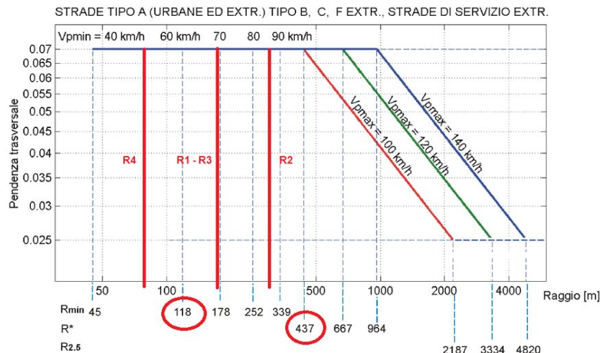
Fig. 13.13: Abacus n. 5.2.4.a, taken from the D.M. 11/05/2001<sup>9</sup>, having the radius of curvature on the x-axis (m), the cross slope on the y-axis (-) for different values of design speeds (V<sub>pmin</sub> = minimum design speed, V<sub>pmax</sub> = maximum design speed). The maximum design speed for this case study is 100 km/h (red diagonal line in the figure).
