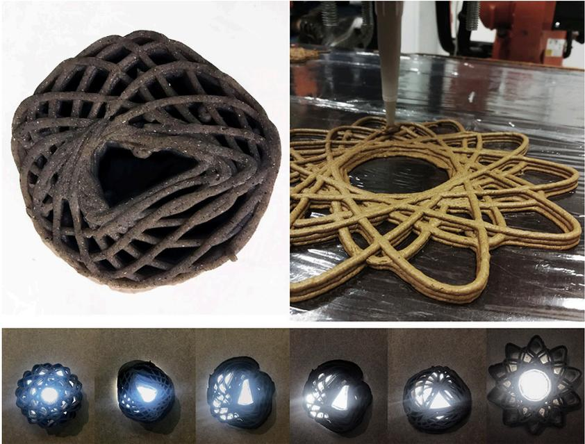
*Fig. 4 - Lifelight; Using digital design and robotic fabrication the team developed a Robotic 3D Printing system for a custom made printable material mixture*
