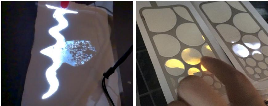
*Fig. 4 - Using water as a replacement for the conductive layer to create samples that encourage new interaction modes*
