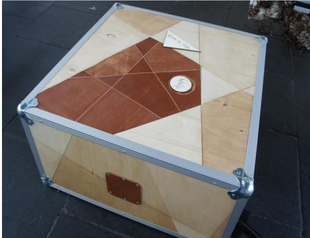
*Fig. 1 - The Sound Box, an interactive sound table that responds to touch by playing different recorded sound files. At the top there is a touch-sensitive surface out of leather and electronic components*
