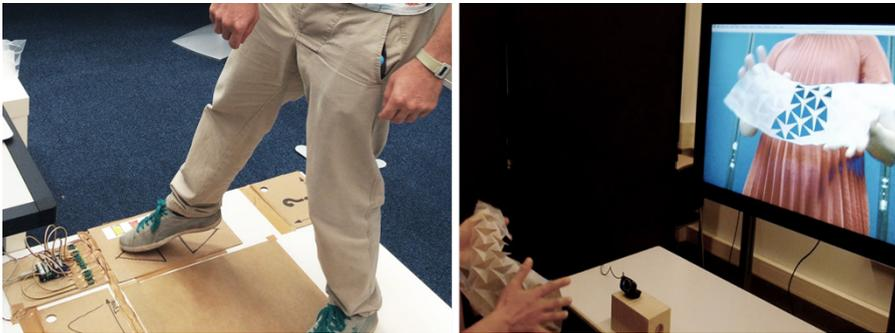
Fig. 3 - Using the input device to control the dynamic behavior of light (left) and the appearance of the real-time Chroma-key effect on the screen (right)
