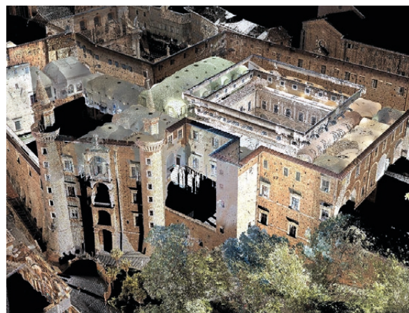
Fig. 2. Point clouds of the Ducal Palace at Urbino.
