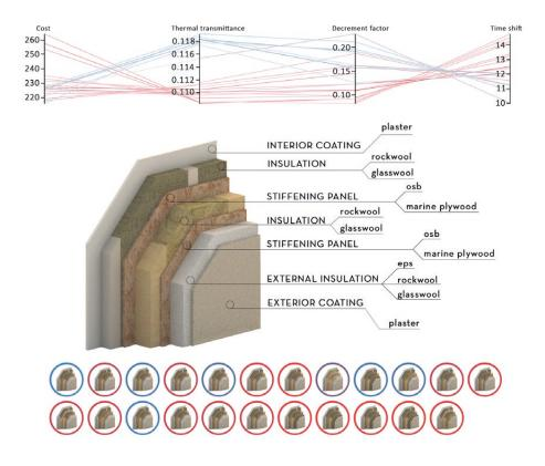
Fig. 1. The selection of various possible optimized walls according to thermal parameters, materials or cost.
