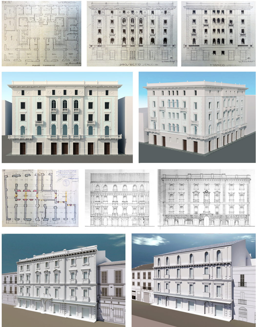
Fig. 1. Some archival documents of two historic buildings in Pescara not built and reworked in 3D.
