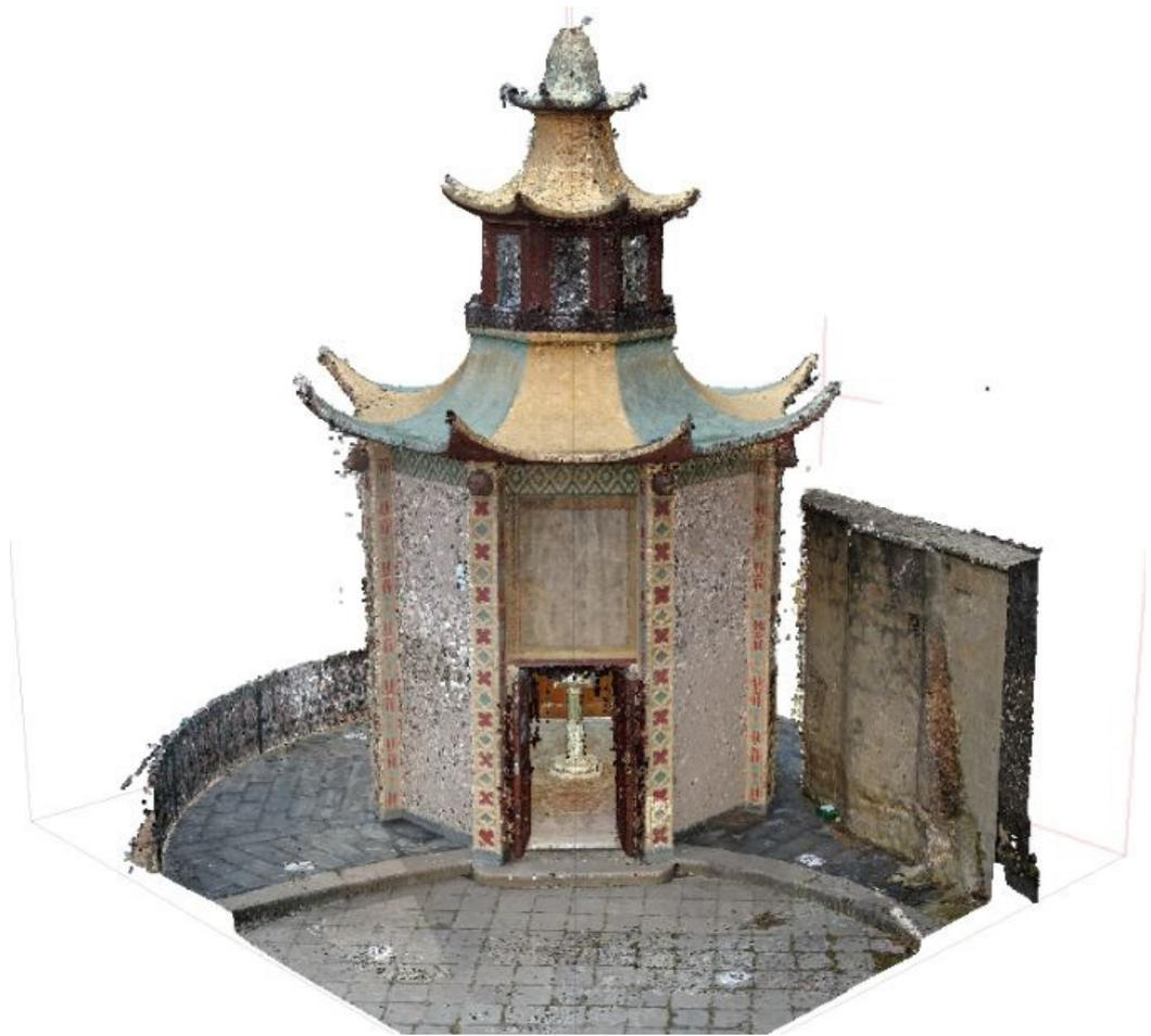
Fig. 03. Point cloud obtained from the aerial photogrammetric survey of the pagoda in Villa Doria d'Angri. Survey and processing by Simona Scandurra.
