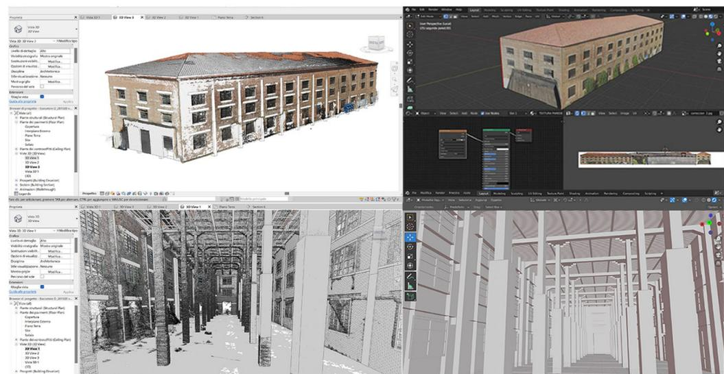
Fig. 06. From point cloud to BIM model, imported in Blender thanks to openBIM extension (author elaboration).
