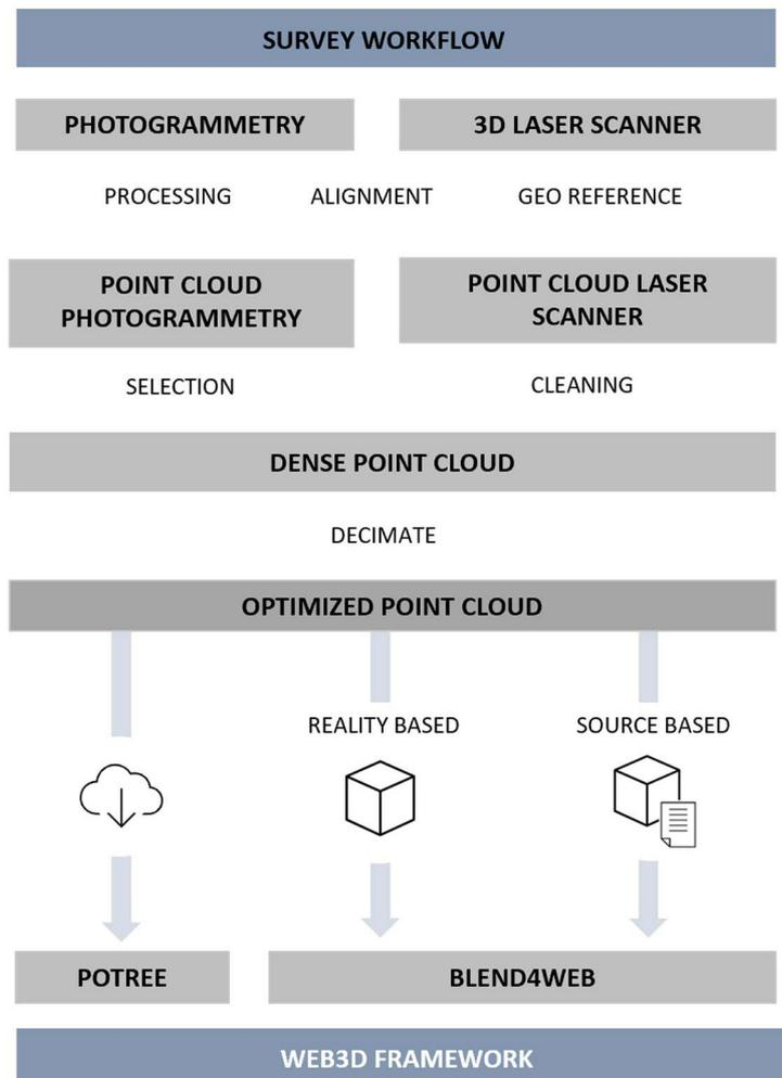
Fig. 04. Schematic workflow from cultural asset acquisition to visualization of 3D content on the Web, illustrating the most appropriate framework based on input data (author elaboration).
