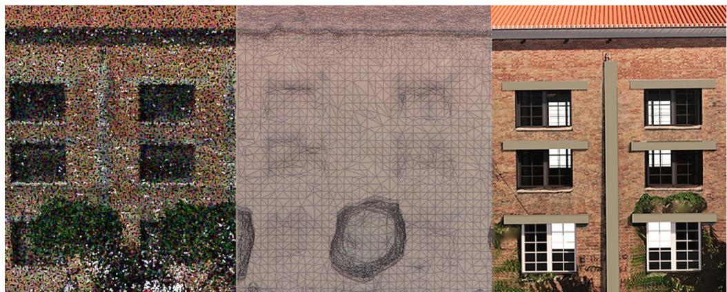
Dense point cloud (left), surface polygonal model (middle) and textured BIM model (right). (Author elaboration).
