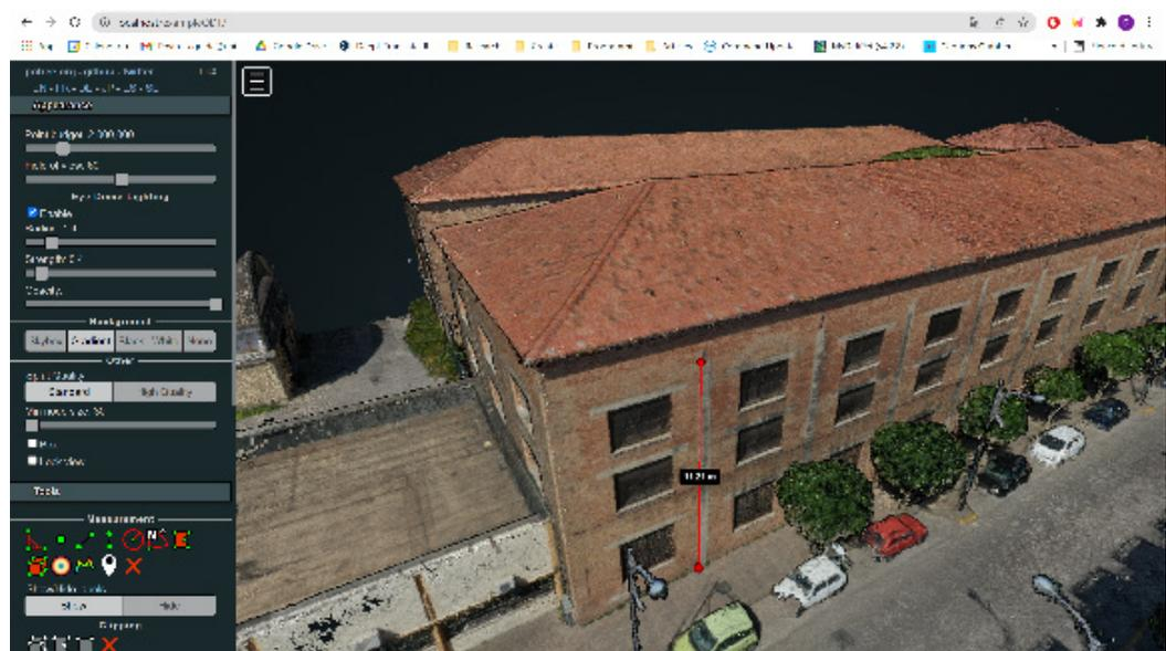
Fig. 05. Potree facilitates basic measurements on the rendered point cloud (author elaboration).
